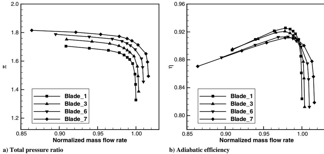
Fig. 2 Operating characteristics of the initialized blades.
