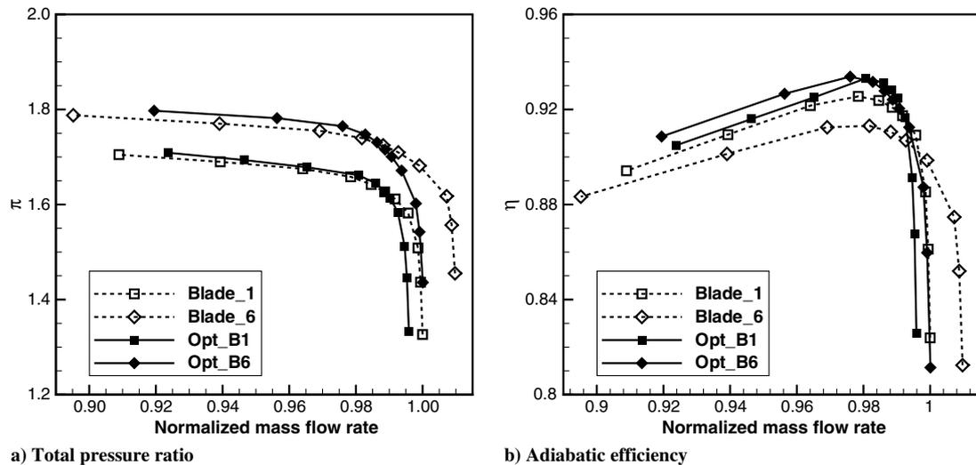
Fig. 5 Operating characteristics of both initialized and optimized blades.
