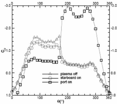
Fig. 2. Comparison of pressure distributions for the plasma off and on at  $\alpha = 40$ ,  $U_\infty = 5$  m/s.
