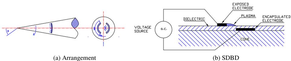
Fig.1. Sketches of the plasma actuators.
