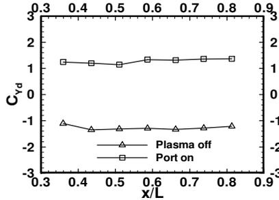
Fig. 3. Local side-force vs.  $x/L$ .
