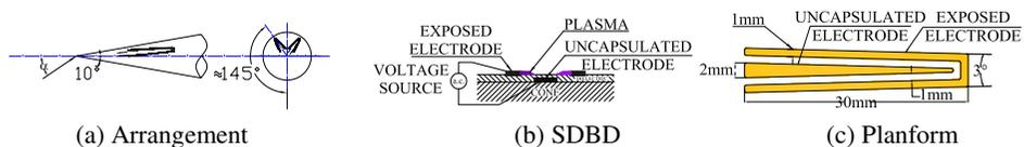
Fig. 1. Sketches of the plasma actuators.
