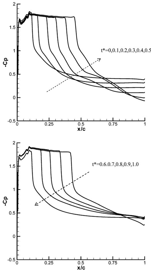
Fig. 12 Unsteady shock movement during one period.
