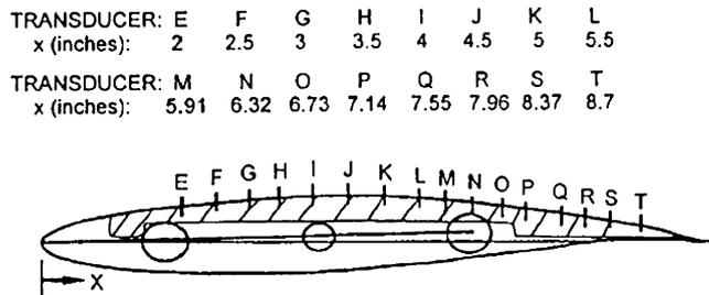
Fig. 1 Geometry of the BGK No. 1 supercritical airfoil (from Ref. 9).
