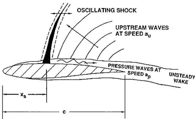
Fig. 13 Model of self-sustained oscillation (from Ref. 12).
