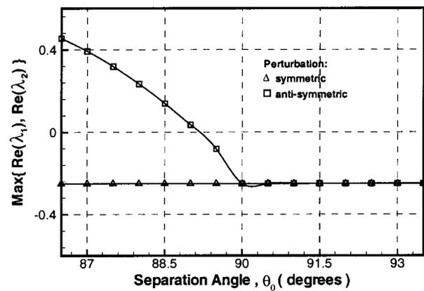
FIG. 11. Maximum real part of eigenvalues of symmetric separation vortex pairs over an elliptic cone vs the (symmetric) separation angle  $\theta_0$ ;  $\tau = c/b = 0.1$ ,  $K = 4$ , and  $K_S = 0$ .
