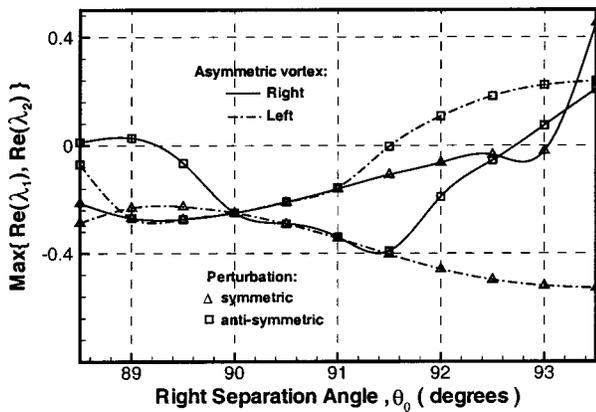
FIG. 12. Maximum real part of eigenvalues of asymmetric separation vortex pairs over an elliptic cone vs the right separation angle  $\theta_0$ ;  $\tau = c/b = 0.1$ , left  $\theta_0 = 90^\circ$ ,  $K = 4$ , and  $K_S = 0$ .
