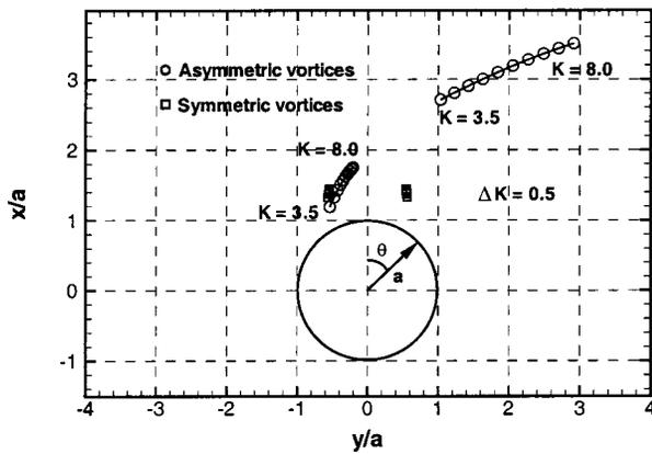
FIG. 5. Location of stationary symmetric and asymmetric vortex pairs over a circular cone for  $K=3.5-8.0$  with a  $0.5$  interval;  $\theta_0=45^\circ$  and  $K_S=0$ .
