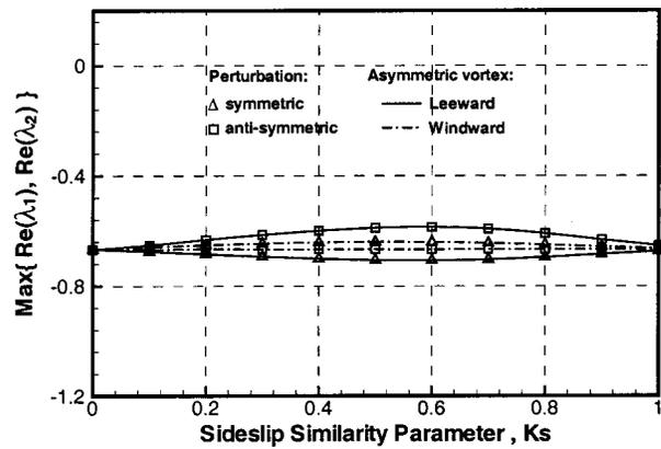
FIG. 3. Maximum real part of eigenvalues of asymmetric vortex pairs over a delta flat-plate wing vs  $K_S$  for  $K = 1.5$ .
