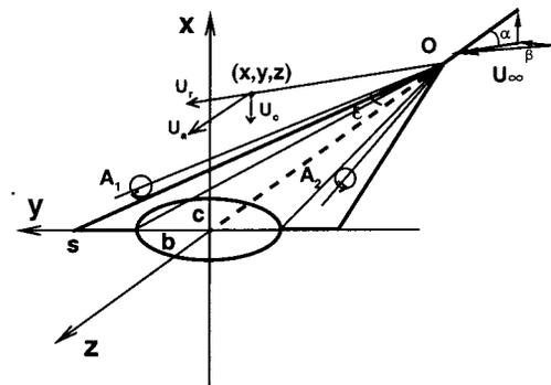
FIG. 1. Slender conical wing-body combination and separation vortices.
