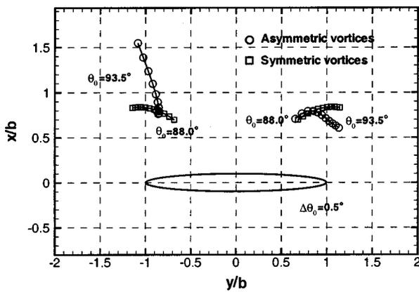
FIG. 10. Location of stationary symmetric and asymmetric separation vortex pairs over an elliptic cone; symmetric vortices are with symmetric separation angles  $\theta_0 = 88.0^\circ - 93.5^\circ$  with a 0.5 interval; asymmetric vortices are with left  $\theta_0 = 90.0^\circ$  and right  $\theta_0 = 88.0^\circ - 93.5^\circ$  with a 0.5 interval;  $\tau = c/b = 0.1$ ,  $K = 4$ , and  $K_S = 0$ .
