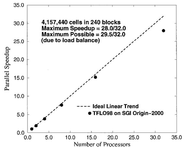
Fig. 4 Parallel performance of TFLO on Origin 2000.
