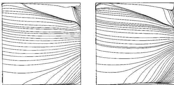
Fig. 11 Predicted limiting streamlines on suction surface of the blade.
