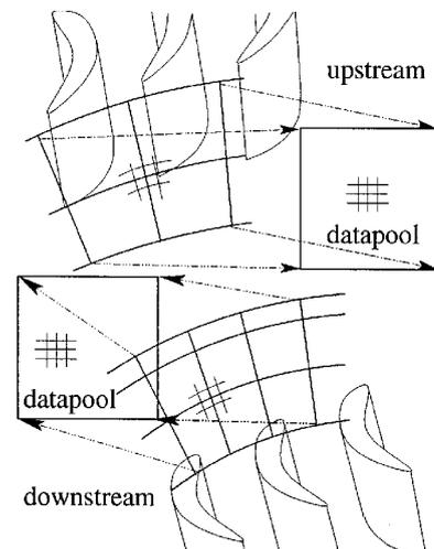
**Fig. 2** Data pools of an inter-blade row interface.
