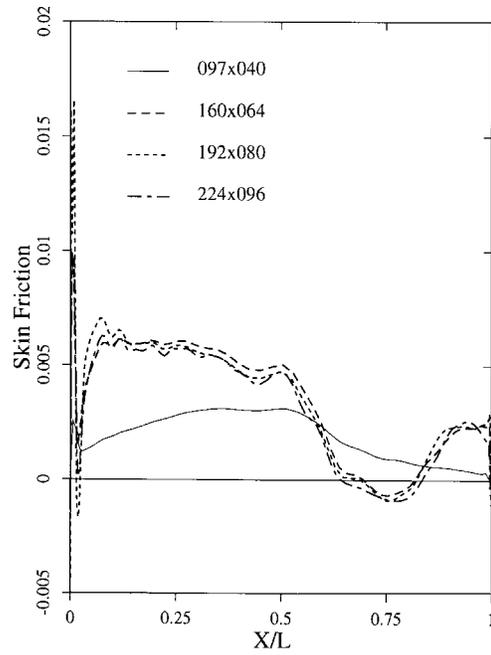
Figure 7. Skin friction obtained on different grids (suction surface, design condition)
