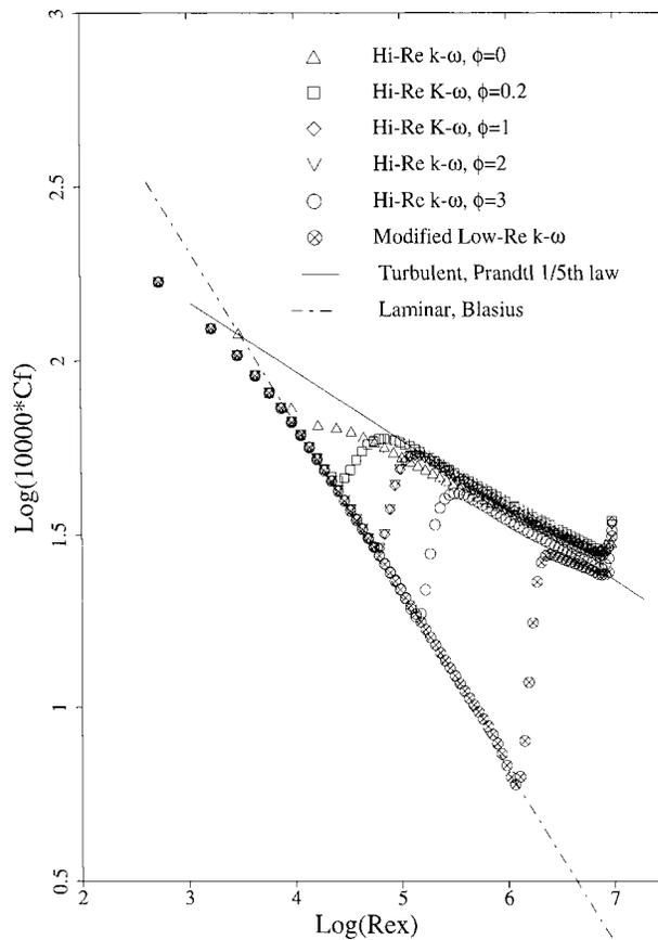
Figure 2. Skin friction coefficients of flat plate flow.  $Re_\infty = 10^7$ , parameter study for  $k-\omega$  models with TSL
