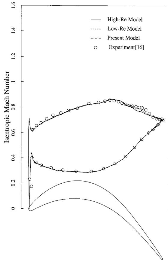
Figure 3. Isentropic Mach number distribution at design condition
