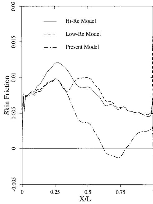
Figure 10. Skin friction coefficient distribution on suction surface, off-design condition
