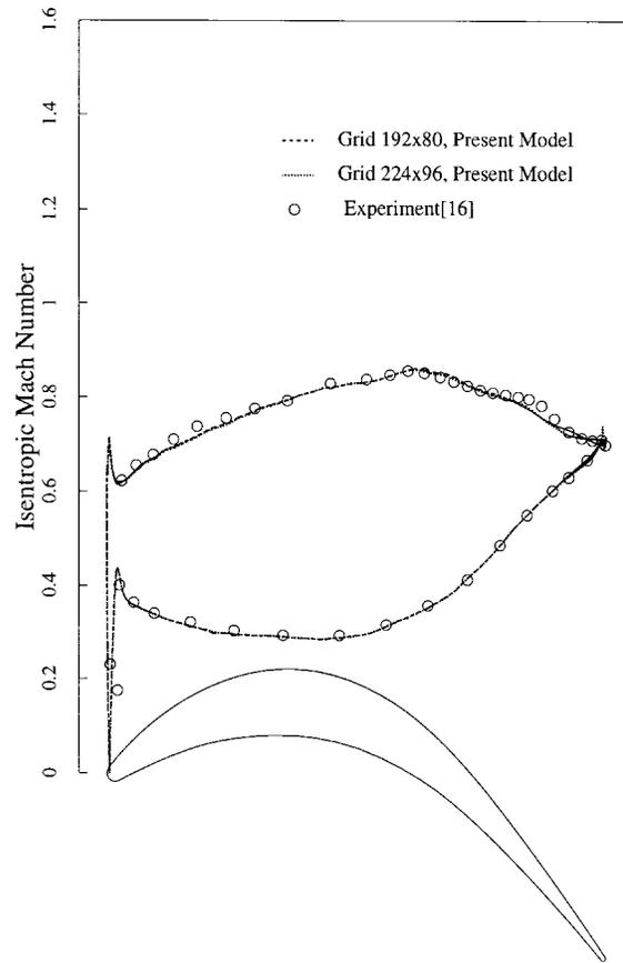
Figure 4. Mesh resolution effects on separation bubble prediction
