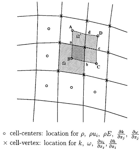
Figure 1. Staggered control volumes for a mixed cell-centre and cell-vertex scheme
