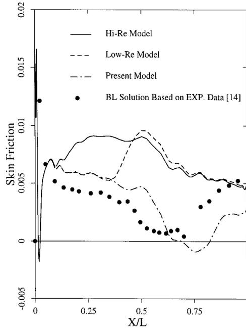
Figure 5. Skin friction coefficient distribution on suction surface, design condition
