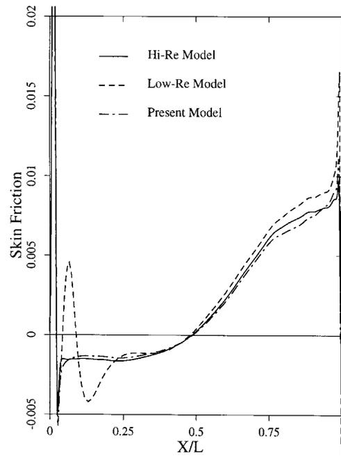
Figure 11. Skin friction coefficient distribution on pressure surface, off-design condition
