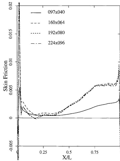
Figure 8. Skin friction obtained on different grids (pressure surface, design condition)
