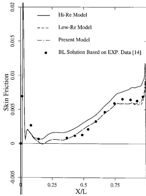
Figure 6. Skin friction coefficient distribution on pressure surface, design condition
