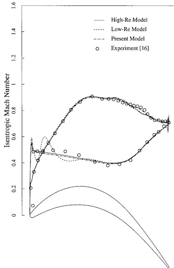
Figure 9. Isentropic Mach number distribution at off-design condition
