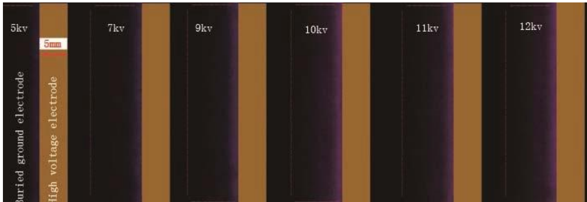
Figure 3. Photograph of NS-DBD F=1.712\text{kHz} , exposure time t=0.04\text{s} containing 68 pulses.
