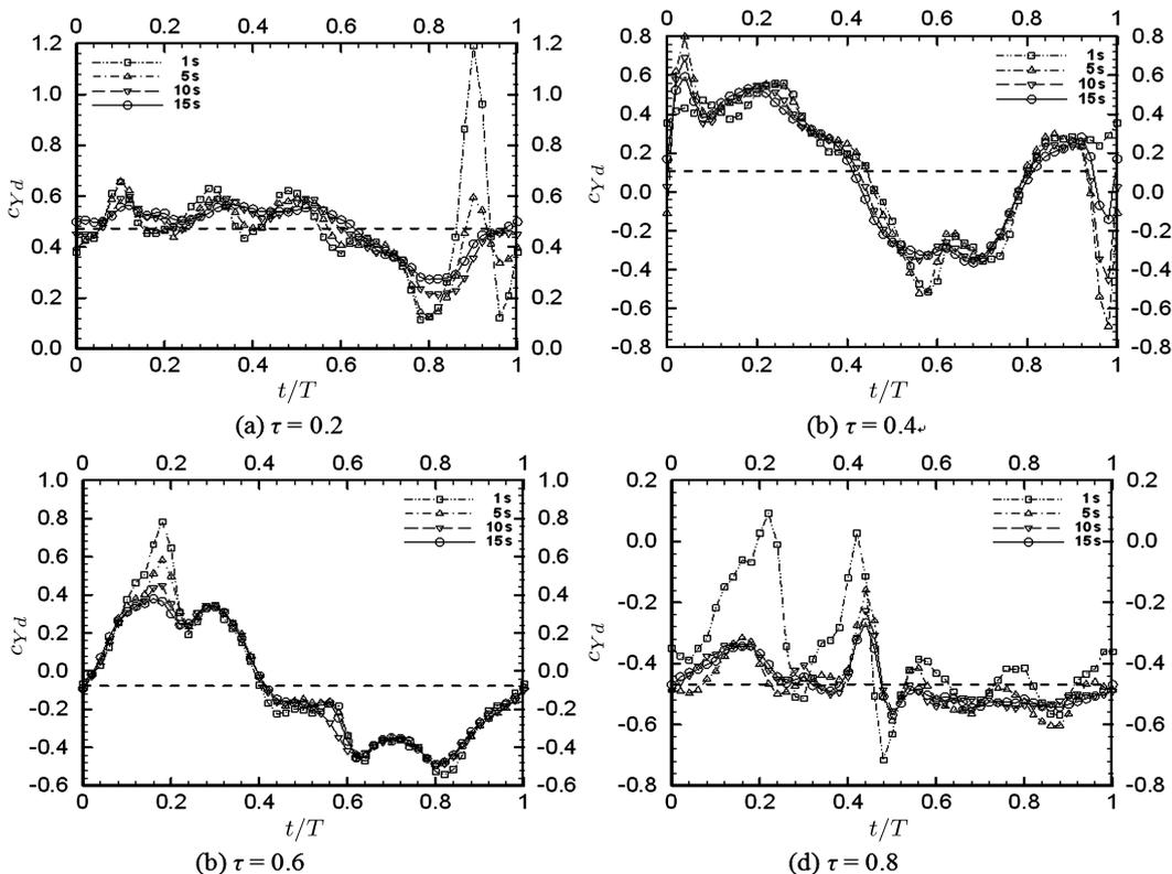
Figure 3: Local side force phase-locked averaged over 1 s-15 s compared with ensemble-averaged side force (dotted line)
