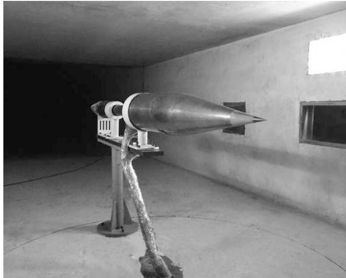
Figure 3. Model in the wind tunnel, leeward view
