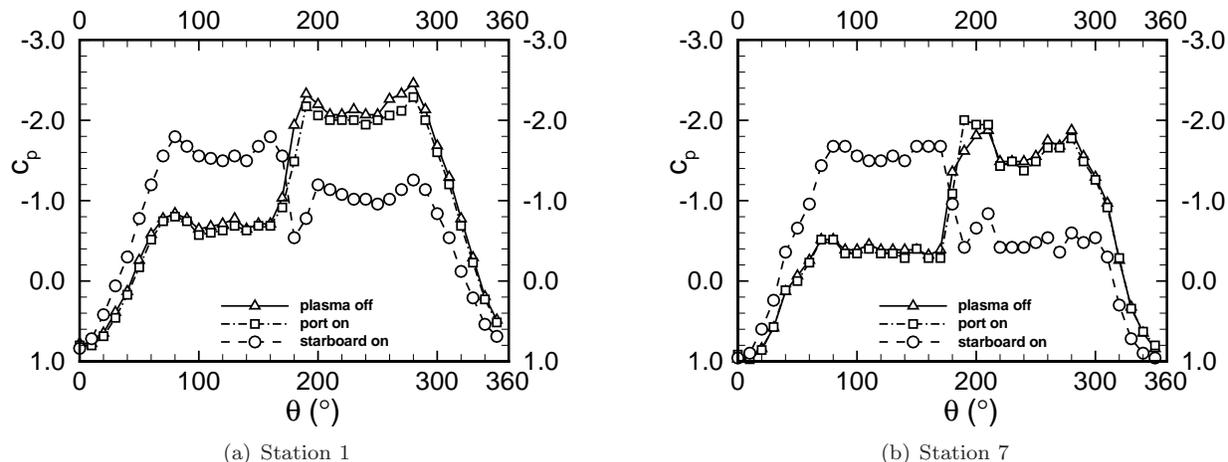
Figure 4. Comparison of pressure distributions for the plasma off and on conditions at  $\alpha = 45^\circ$ .
