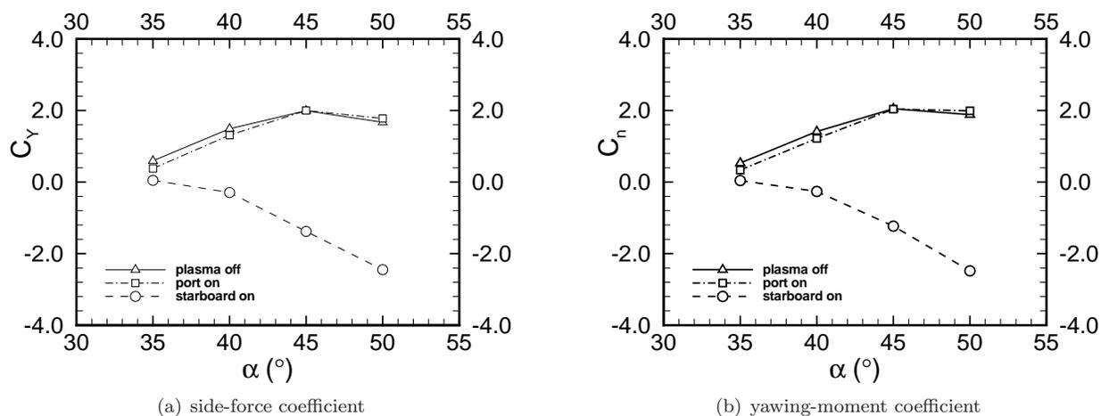
Figure 3. Side forces and yawing moments vs. angle of attack for plasma on and off conditions.
