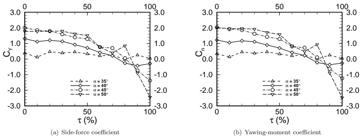
Figure 5. Side force and yawing moment on the cone produced by duty-cycled plasma control.
