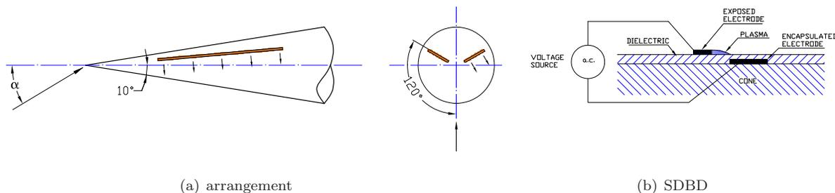
**Figure 1. Sketches of the plasma actuators.**
