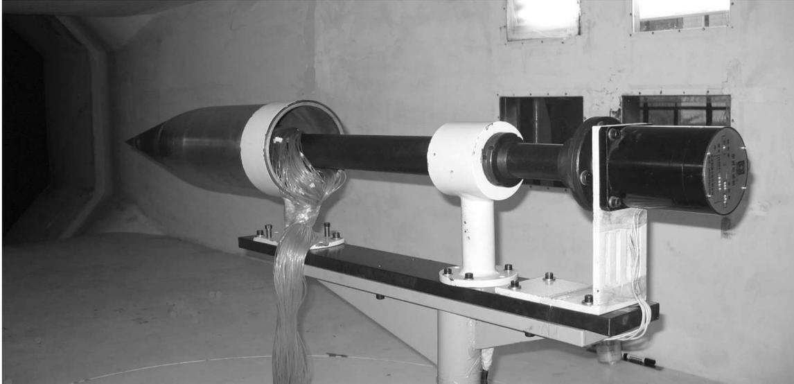
(a) model in the wind tunnel
