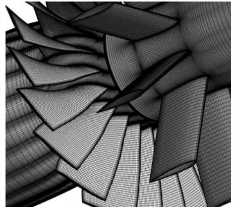
Figure 5 Grid of IGV/Rotor (Rotor 67)
