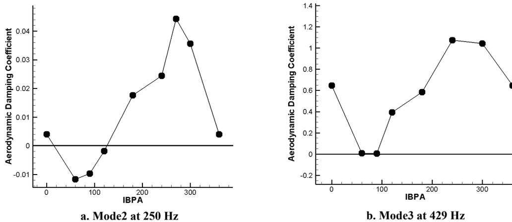
Figure 7 Unsteady results of Rotor 67: aerodynamic damping coefficients - IBPA
