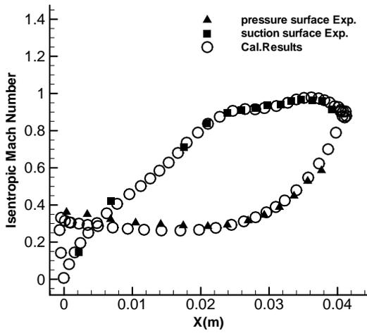
Figure 1 Steady results of STCF4 (Case 552B)
