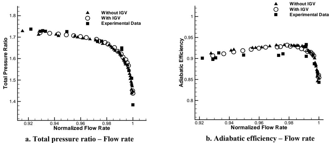
Figure 6 Steady results of Rotor 67: performance map
