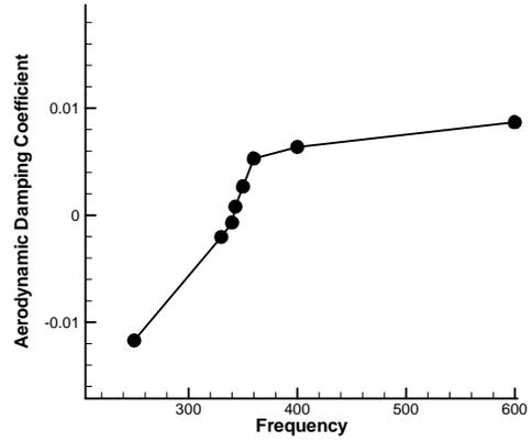
Figure 8 Aerodynamic damping coefficients – frequency: Mode 2, IBPA=60°
