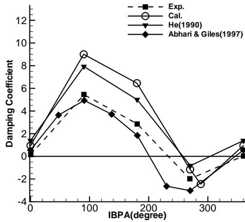
Figure 2 Unsteady results of STCF4: aerodynamic damping coefficient vs. IBPA (Case 552B)
