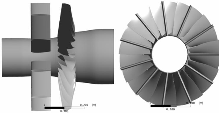
Figure 4 Different views of the IGV/Rotor model (Rotor 67)
