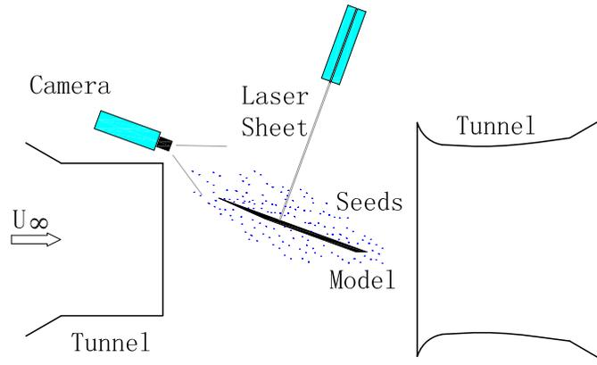
Figure 6. Schematic of the PIV experimental setup.
