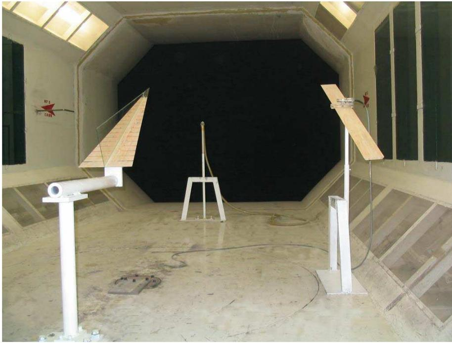
Figure 2. Photograph of the test section layout for smoke-laser-sheet experiments.
