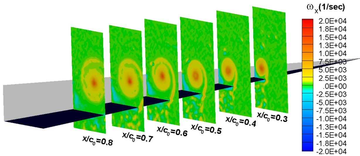
Figure 9. Contours of the time-averaged axial vorticity of the starboard vortex on the cross-sections  $x/c_0 = 0.3 - 0.8$  for the wing+0.6s-fin model at  $\alpha = 30^\circ$ ,  $\beta = 0$ .
