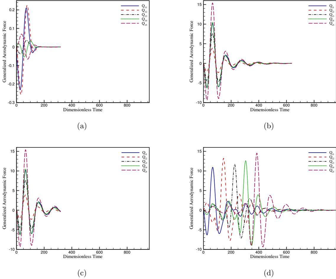
Figure 2. (a) Response of system with mode by mode input, in this case FIM was prescribed to mode 1. (b) Response of system with simultaneous input of FIM signals. (c) Truncated version of simultaneous input. (d) Staggered sequence of FIM signals.
