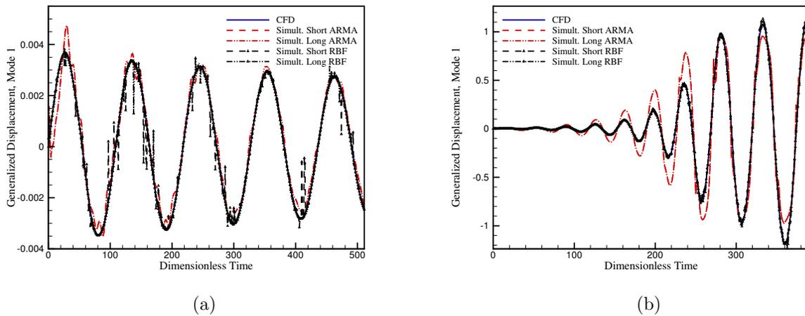
Figure 7. (a) Time history of the generalized coordinates for the AGARD 445.6 wing for  $M_\infty = 0.96$  and  $V_f = 0.2$ , by ARMA and RBF trained on simultaneous FIM inputs. (b)  $M_\infty = 1.141$  and  $V_f = 0.75$ .
