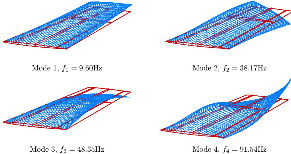
Figure 6. Modal shape deflections and frequencies for the 445.6 wing (weakened model). Only alternate mesh lines have been shown.
