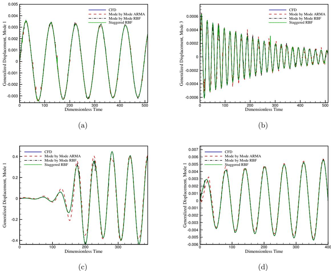
**Figure 11.** (a) Time history of the generalized coordinates for the AGARD 445.6 wing for  $M_\infty = 0.96, V_f = 0.25$ , mode 1, by ARMA and RBF trained on mode by mode and staggered FIM inputs. (b)  $M_\infty = 0.85, V_f = 0.30$ , mode 3. (c)  $M_\infty = 0.85, V_f = 0.50$ , mode 1. (d)  $M_\infty = 0.678, V_f = 0.42$ , mode 1.
