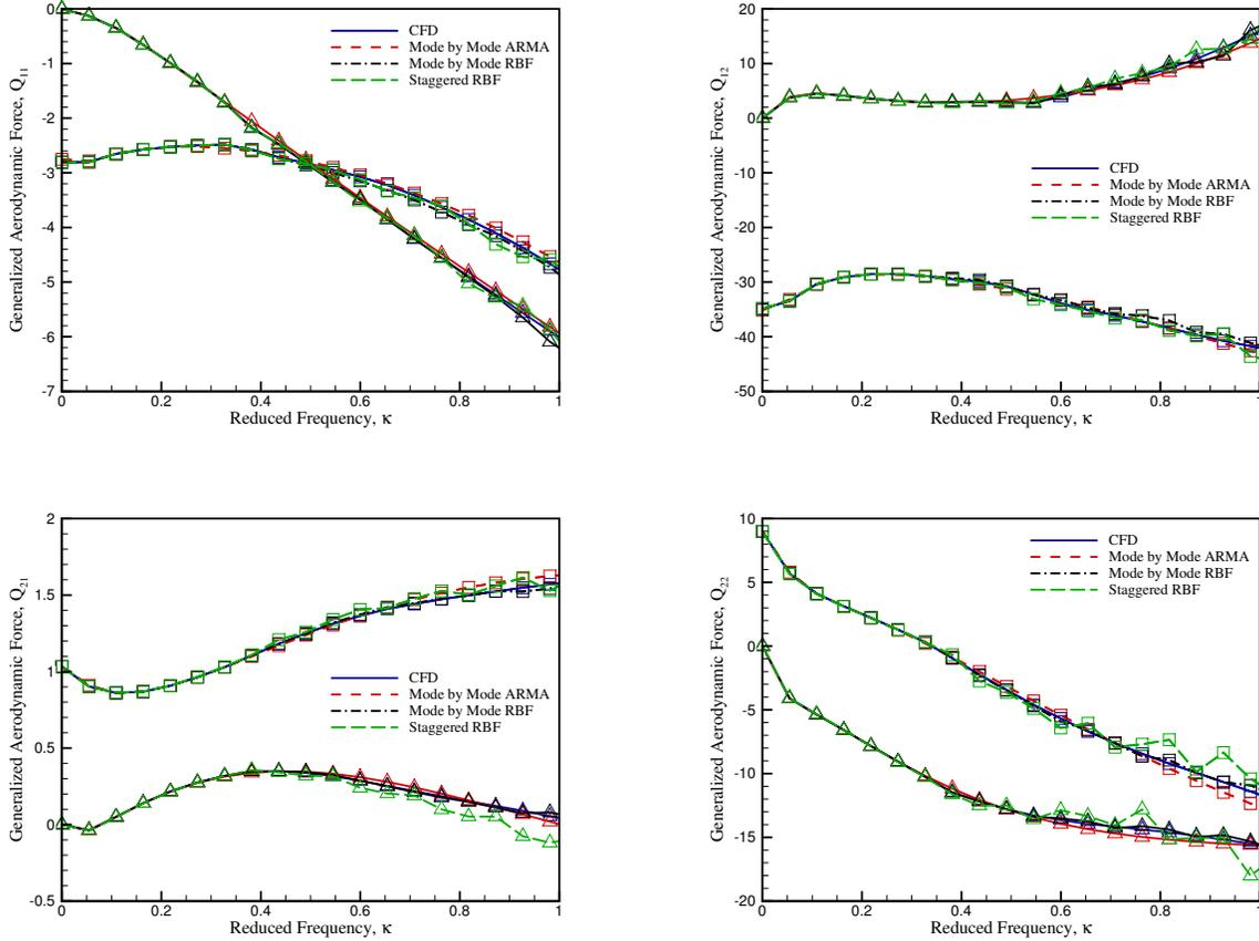
Figure 10. Generalized aerodynamic force  $Q_{11}$ ,  $Q_{12}$ ,  $Q_{21}$ , and  $Q_{22}$  for  $M_\infty = 0.960$ . Models trained via mode by mode and staggered input of FIM.  $\square$  denotes real part,  $\triangle$  denotes imaginary part.
