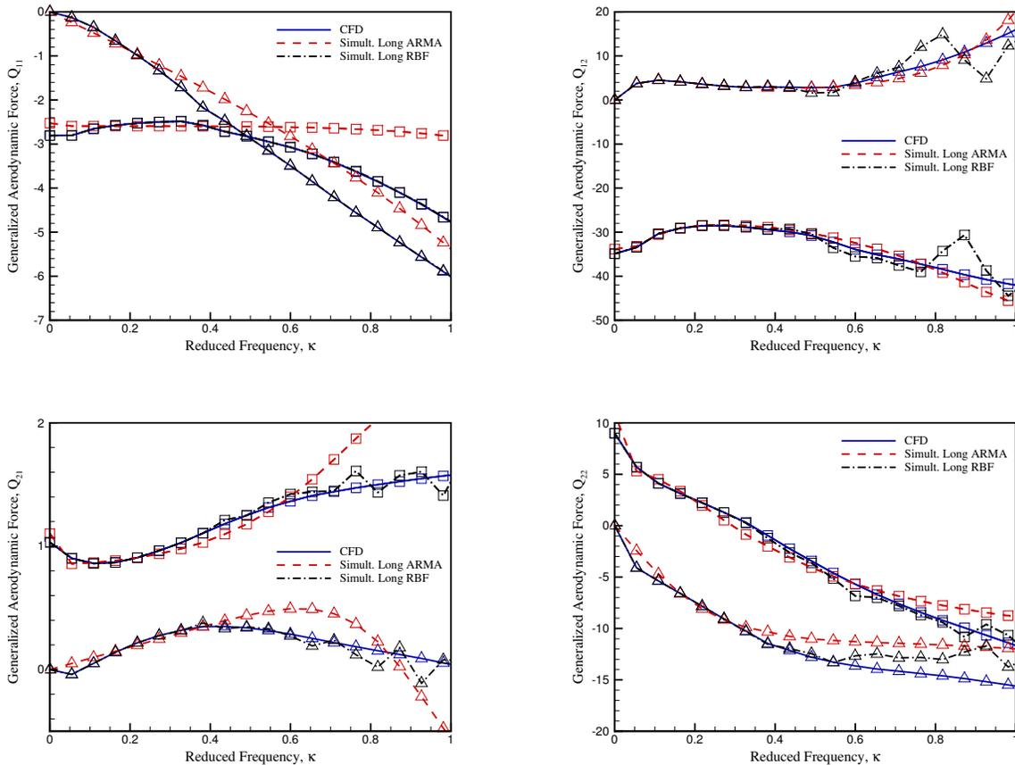
**Figure 9. Generalized aerodynamic force  $Q_{11}$ ,  $Q_{12}$ ,  $Q_{21}$ , and  $Q_{22}$  for  $M_\infty = 0.960$ . Models trained via simultaneous input of FIM.  $\square$  denotes real part,  $\triangle$  denotes imaginary part.**
