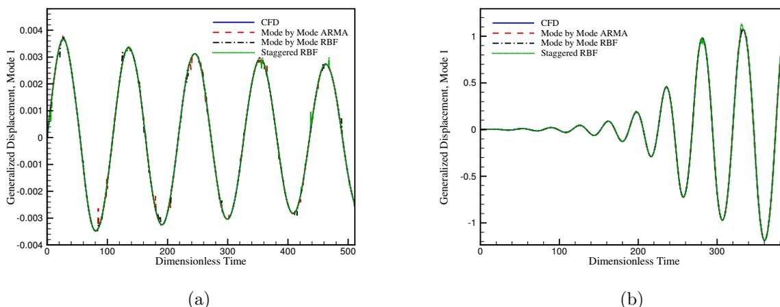
**Figure 8.** (a) Time history of the generalized coordinates for the AGARD 445.6 wing for  $M_\infty = 0.96$  and  $V_f = 0.2$ , by ARMA and RBF trained on mode by mode and staggered FIM inputs. (b)  $M_\infty = 1.141$  and  $V_f = 0.75$ .
