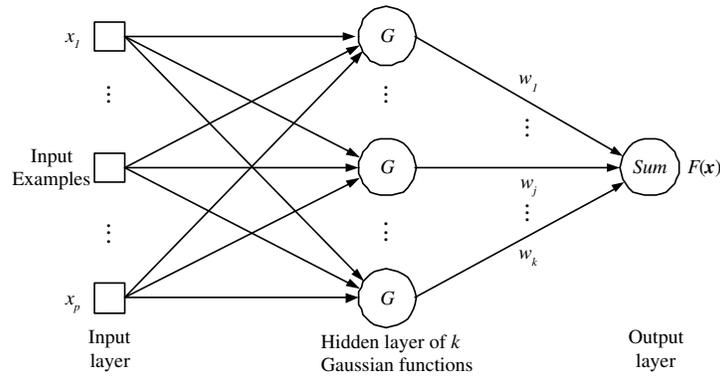
Figure 3. Schematic diagram of the Radial Basis Functions (RBF) network.
