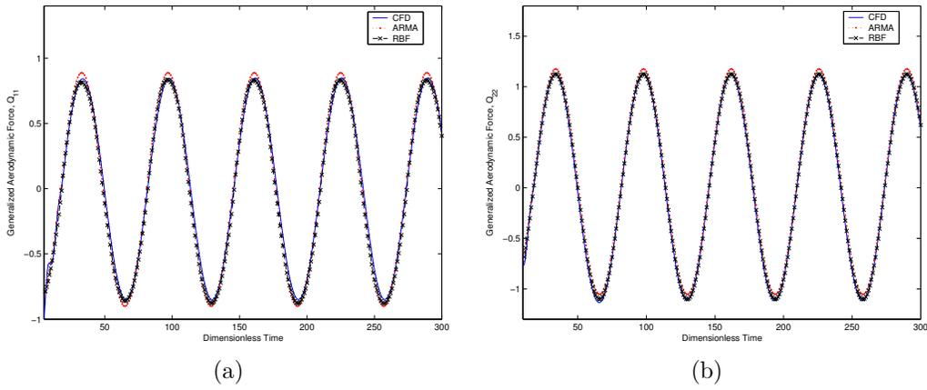
Figure 4. (a) Prediction of  $Q_{11}$  via training of mode by mode. (b) Prediction of  $Q_{22}$  via training of combined signal.
