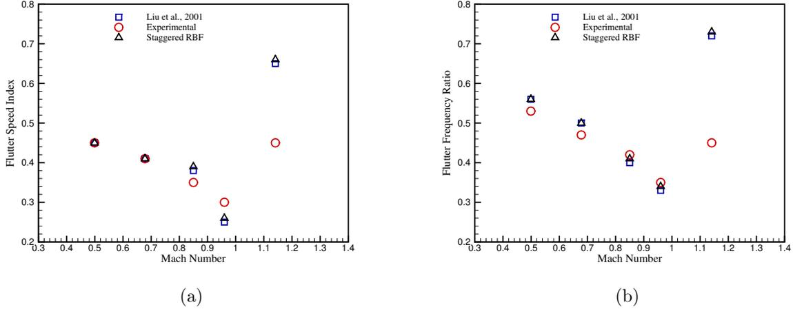
Figure 12. (a) Flutter speed for the AGARD 445.6 wing. (b) Flutter frequency for the AGARD 445.6 wing.
