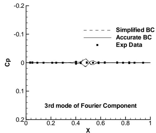
Fig. 12 Comparison of computational surface pressure distribution of NACA64A010 with experimental data,  $M_\infty = 0.796$ ,  $\alpha_m = 0.0$  degrees,  $\alpha_0 = 1.01$  degrees,  $\kappa = 0.202$  (Real part) .
