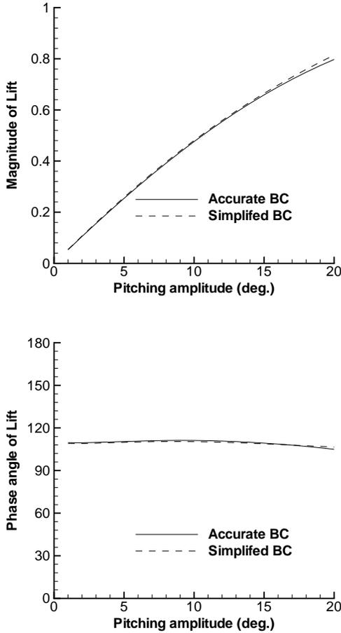
Fig. 14 Comparison of first mode of lift coefficients versus the amplitude of the pitching for NACA64A010,  $M_\infty = 0.796$ ,  $\kappa = 0.202$ .
