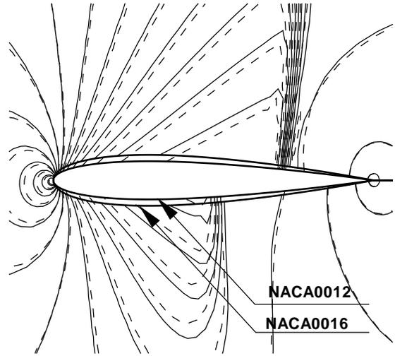
Fig. 4 Pressure contours for NACA0016,  $M_\infty = 0.80$ ,  $\alpha = 2.0$  degrees (Solid lines represent the results with accurate boundary conditions and dash lines represent results with simplified boundary conditions).
