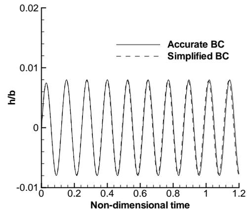
Fig. 15 Time history of pitching and plunging motion for Isogai wing model for  $M_\infty = 0.750$ ,  $V_f = 1.00$ .
