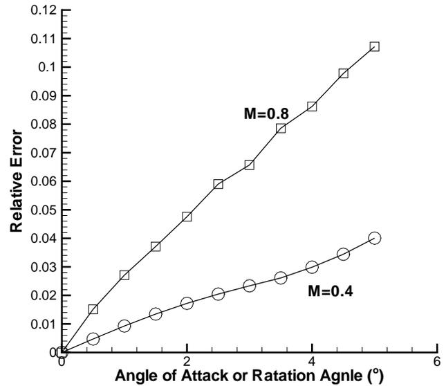
Fig. 11 Relative error versus the rotation angle of NACA0012.
