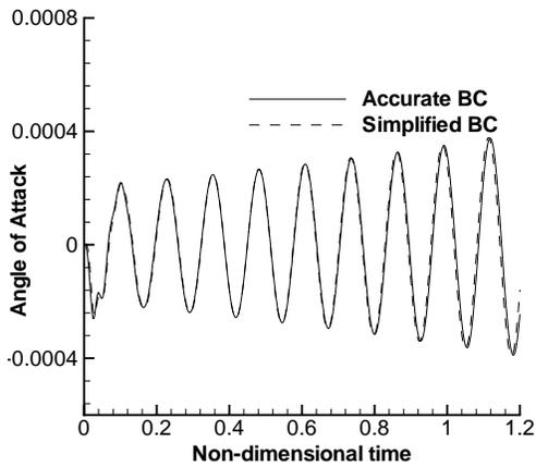
Fig. 17 Time history of pitching and plunging motion for Isogai wing model for  $M_\infty = 0.750$ ,  $V_f = 1.20$ .
