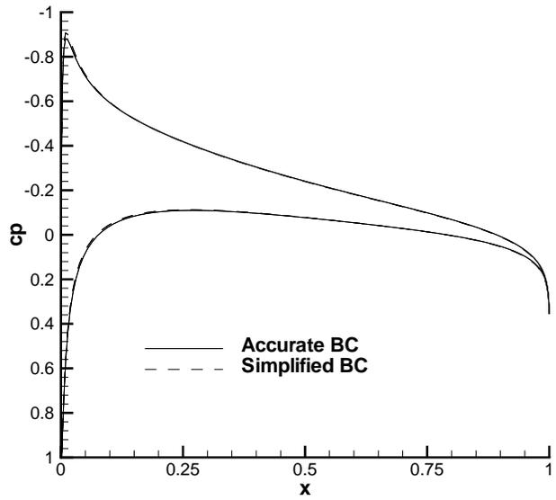
Fig. 3 Pressure distribution for NACA0008 with different grids and boundary conditions  $M_\infty = 0.40$ ,  $\alpha = 2.0$  degrees.
