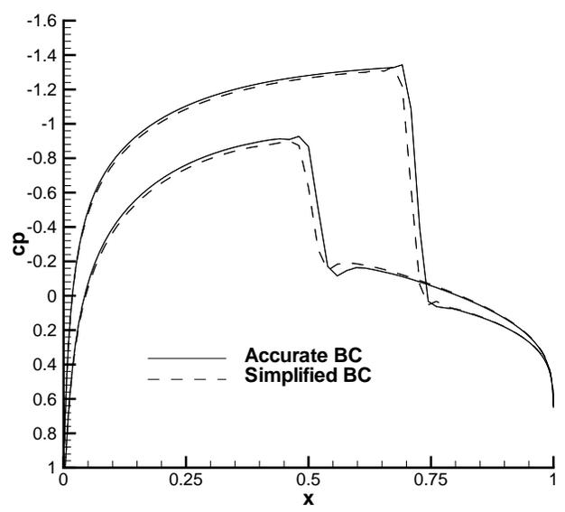
Fig. 5 Pressure distribution for NACA0016,  $M_\infty = 0.80$ ,  $\alpha = 2.0$  degrees.
