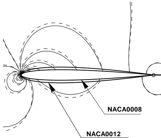
Fig. 2 Pressure contours for NACA0008 with different grids and boundary conditions,  $M_\infty = 0.40$ ,  $\alpha = 2.0$  degrees (Solid lines represent the results with accurate boundary conditions and dash lines represent results with simplified boundary conditions).
