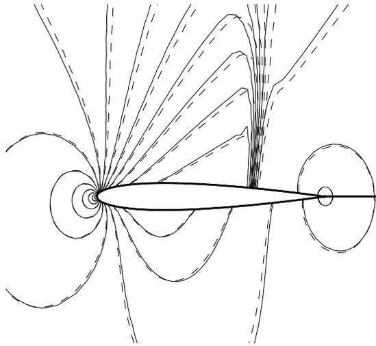
Fig. 9 Pressure contours for NACA0012,  $M_\infty = 0.80$ ,  $\alpha=2.0$  degrees (Solid lines represent the results with accurate boundary conditions and dash lines represent results with simplified boundary conditions).
