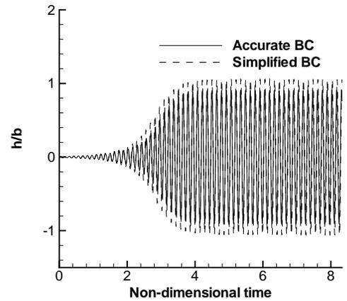
Fig. 19 Time history of pitching and plunging motion for Isogai wing model for  $M_\infty = 0.750$ ,  $V_f = 1.33$ .
