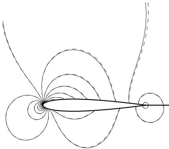
Fig. 7 Pressure contours for NACA0012,  $M_\infty = 0.40$ ,  $\alpha = 2.0$  degrees (Solid lines represent the results with accurate boundary conditions and dash lines represent results with simplified boundary conditions).
