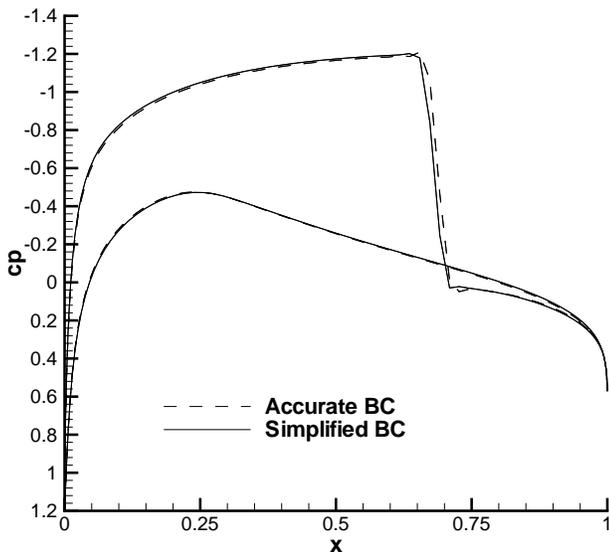
Fig. 10 Pressure distribution for NACA0012,  $M_\infty = 0.80$ ,  $\alpha=2.0$  degrees.
