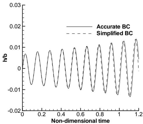
Fig. 18 Comparison of flutter boundary of NACA64A010.
