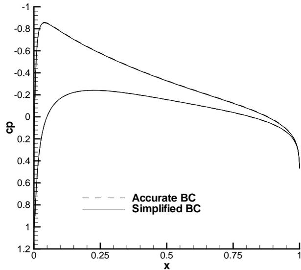
Fig. 8 Pressure distribution for NACA0012,  $M_\infty = 0.40$ ,  $\alpha = 2.0$  degrees.
