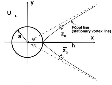
Fig. 7 Circular cylinder with a rear splitter plate.
