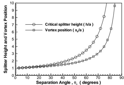
Fig. 9 Vortex position and critical height of splitter plate as function of separation angle for circular cylinder with a splitter plate.
