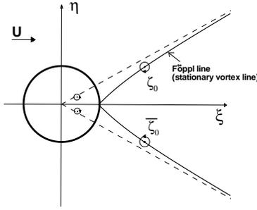
**Fig. 1 Vortices behind a Circular Cylinder and Föpl Line.**
