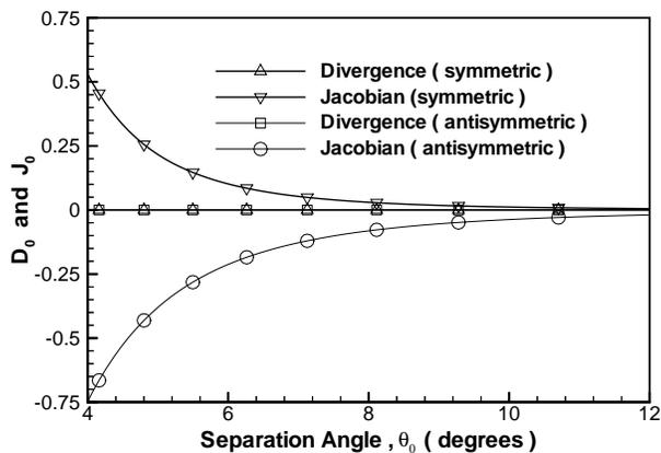
**Fig. 16 Divergence and Jacobian vs. separation angle for an elliptic cylinder,  $\tau = 6.0$ .**
