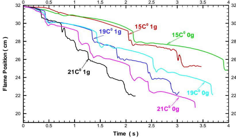
Figure 2: Flame location versus time after ignition.
