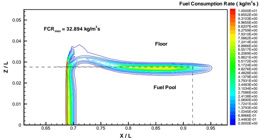
Figure 9: Contours of fuel consumption rate in the  $x$ - $z$  plane at  $y = 1 \text{ mm}$ ,  $t = 1.63\text{s}$ , Case 1A.
