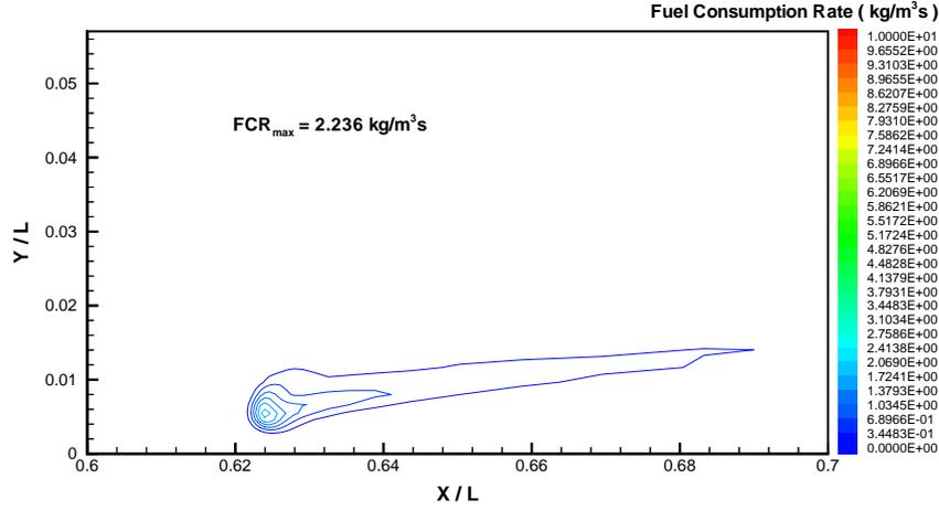
Figure 21: Contours of fuel consumption rate in the  $x$ - $y$  plane at  $z/L = 0.0$ ,  $t = 2.65s$ , Case 1B.
