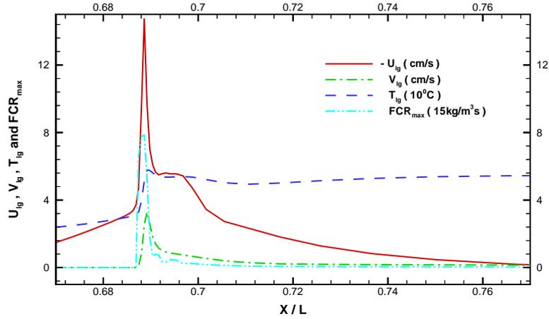
Figure 19: Flow velocity, temperature, fuel vapor vertical velocity at the fuel-air interface, and maximum fuel consumption rate (searched along  $y$  direction) versus  $x$  at  $z/L = 0.0$ ,  $t = 2.08s$ , Case 1B.
