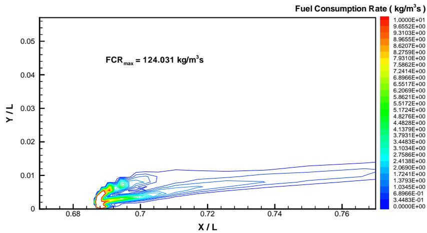
Figure 5: Contours of fuel consumption rate in the  $x$ - $y$  symmetry plane at  $z/L = 0.0$ ,  $t = 1.63\text{s}$ , Case 1A.
