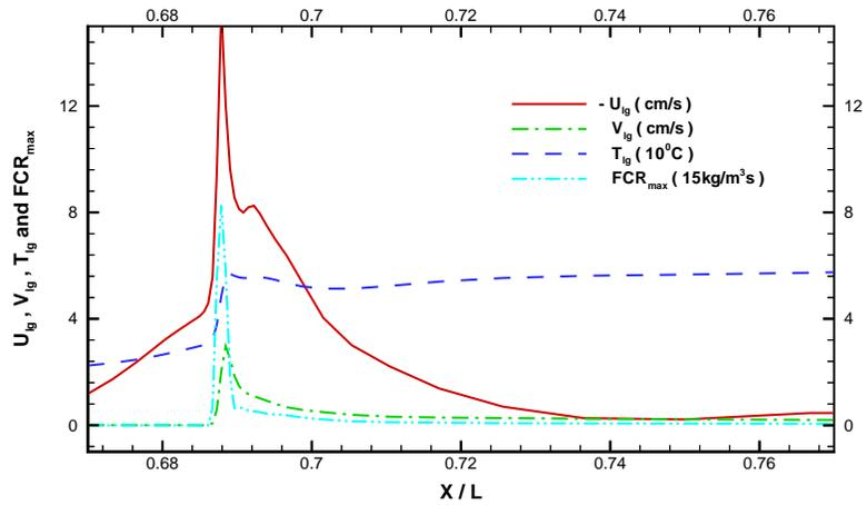
Figure 8: Flow velocity, temperature, fuel vapor vertical velocity at the fuel-air interface, and maximum fuel consumption rate at  $z/L = 0.0$ ,  $t = 1.63s$ , Case 1A.
