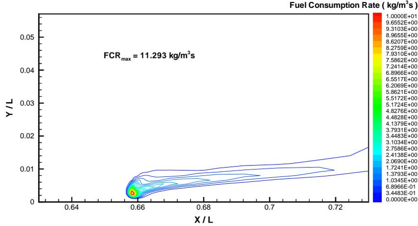
Figure 14: Contours of fuel consumption rate in the  $x$ - $y$  symmetry plane at  $z/L = 0.0$   $t = 1.87s$ , Case 1A.
