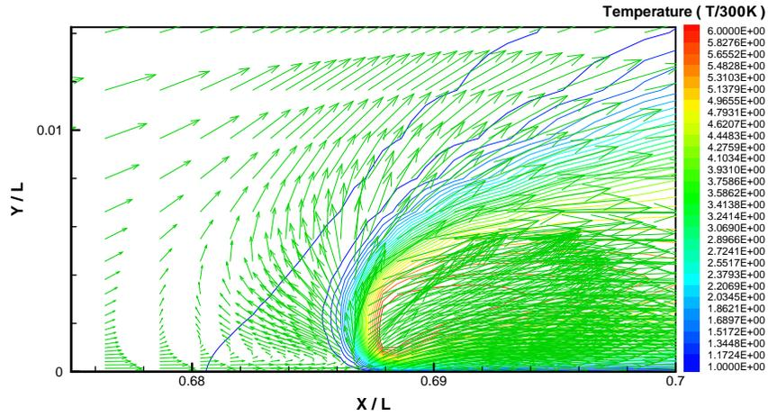
Figure 7: Contours of temperature and relative velocity vectors in the  $x$ - $y$  symmetry plane at  $z/L = 0.0$ ,  $t = 1.63s$ , Case 1A.
