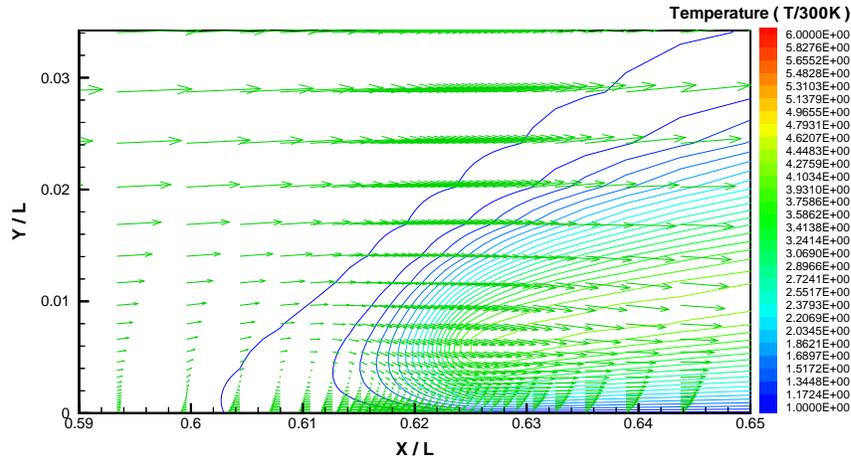
Figure 22: Relative velocity vectors and temperature contours in the  $x$ - $y$  plane at  $z/L = 0.0$ ,  $t = 2.65s$ , Case 1B.
