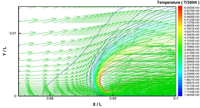
Figure 18: Relative velocity vector and contours of temperature in the  $x$ - $y$  symmetry plane at  $z/L = 0.0$ ,  $t = 2.08s$ , Case 1B.
