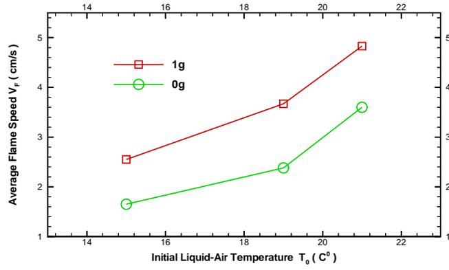
Figure 3: Average flame speed versus initial fuel-air temperature
