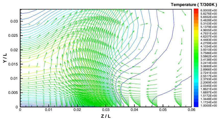
Figure 13: Velocity vector and contours of temperature in the  $z$ - $y$  plane at  $x/L = 0.788$ ,  $t = 1.63\text{s}$ , Case 1A.
