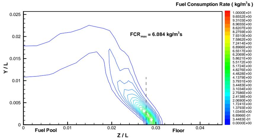
Figure 12: Contours of fuel consumption rate in the  $z$ - $y$  plane at  $x/L = 0.788$ ,  $t = 1.63\text{s}$ , Case 1A.
