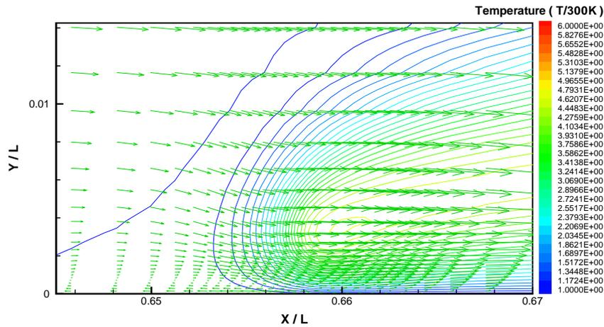
Figure 15: Relative velocity vectors and temperature contours in the  $x$ - $y$  symmetry plane at  $z/L = 0.0$   $t = 1.87s$ , Case 1A.
