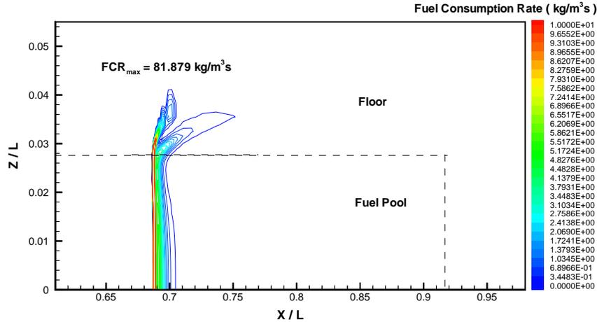
Figure 20: Contours of fuel consumption rate in the  $x$ - $z$  plane at  $y = 1$  mm,  $t = 2.08s$ , Case 1B.
