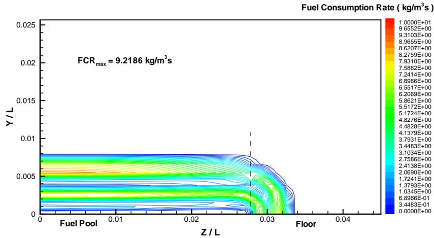
Figure 10: Contours of fuel consumption rate in the  $z$ - $y$  plane at  $x/L = 0.691$ ,  $t = 1.63\text{s}$ , Case 1A.
