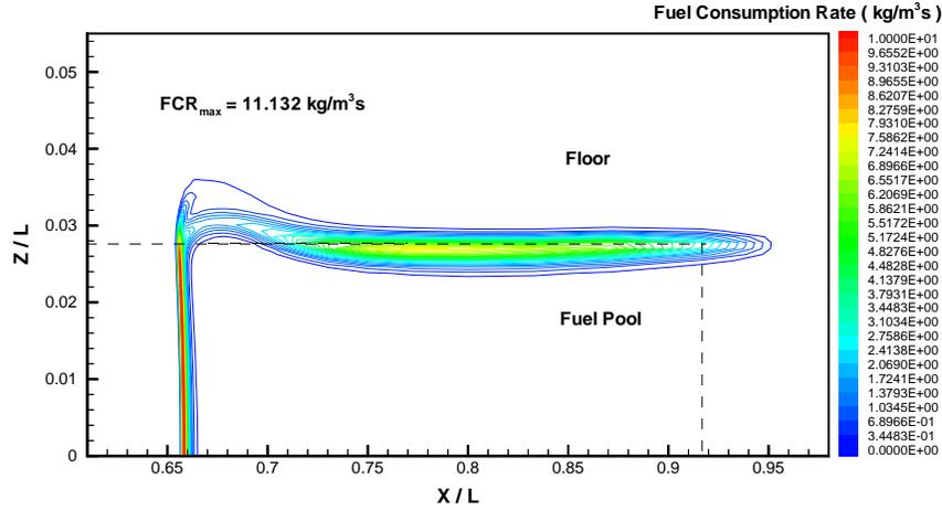
Figure 16: Contours of fuel consumption rate in the  $x$ - $z$  plane at  $y = 1$  mm,  $t = 1.87$ s, Case 1A.
