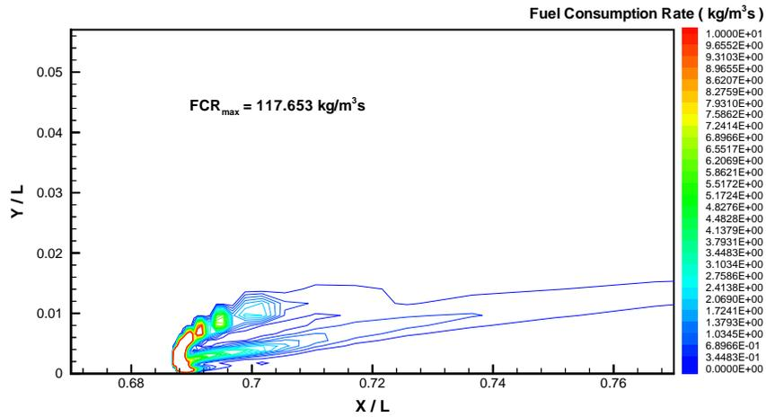
Figure 17: Contours of fuel consumption rate in the  $x$ - $y$  plane at  $z/L = 0.0$ ,  $t = 2.08$ s, Case 1B.
