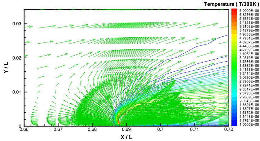
Figure 6: Contours of temperature and velocity vectors in the  $x$ - $y$  symmetry plane at  $z/L = 0.0$ ,  $t = 1.63s$ , Case 1A.
