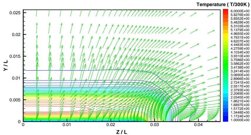
Figure 11: Velocity vector and contours of temperature in the  $z$ - $y$  plane at  $x/L = 0.691$ ,  $t = 1.63\text{s}$ , Case 1A.
