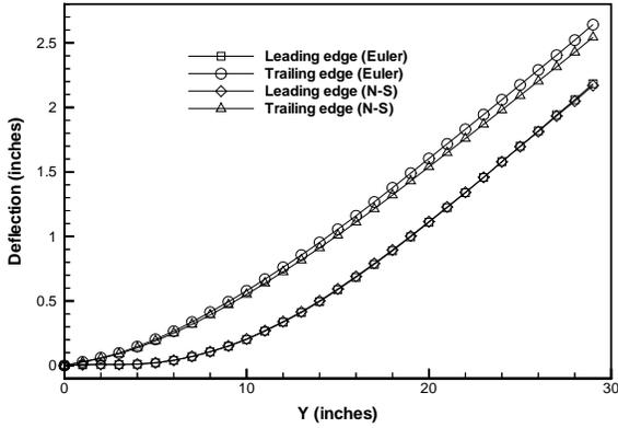
Fig. 20 Vertical deflection of wing along span relative to the wing root
