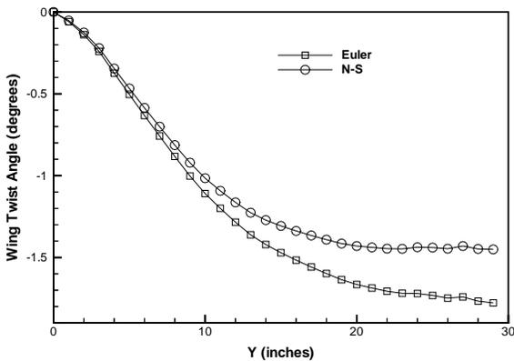
Fig. 21 Twist of wing along span relative to the wing root
