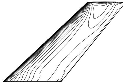
Fig. 19 Pressure contours on lower surface of elastic wing, Navier-Stokes solution
