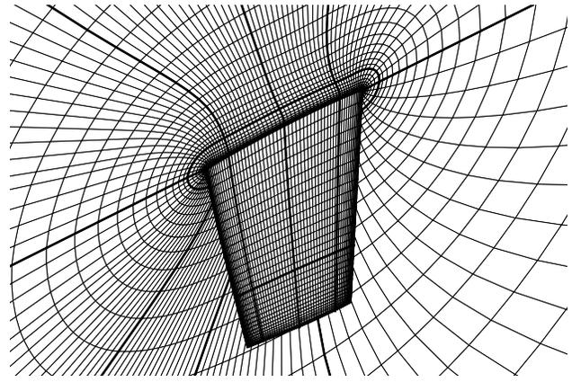
Fig. 2 Perspective view of the O-grid. The thick lines show the block boundaries. The off-body grid is at the plane of symmetry.
