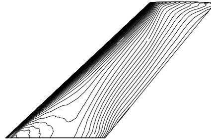
Fig. 18 Pressure contours on upper surface of elastic wing, Navier-Stokes solution
