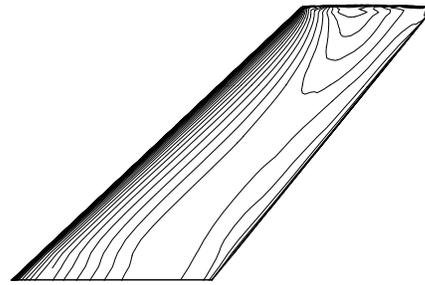
Fig. 11 Pressure contours on lower surface of rigid wing, Euler solution
