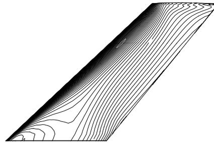
Fig. 12 Pressure contours on upper surface of rigid wing, Navier-Stokes solution
