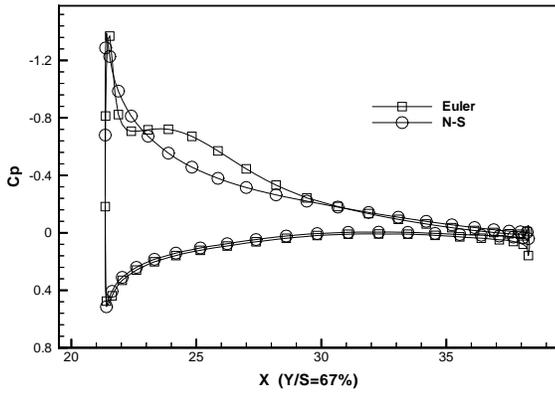
Fig. 9 Comparison of  $C_p$  distributions at 67% span by Euler and Navier-Stokes equations for the rigid wing
