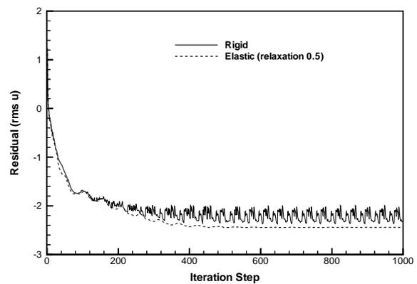
Fig. 7 Comparison of convergence histories for rigid and elastic wings, Navier-Stokes computation
