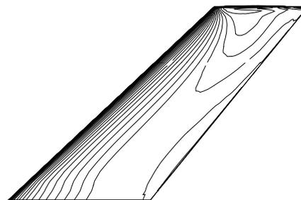
Fig. 13 Pressure contours on lower surface of rigid wing, Navier-Stokes solution
