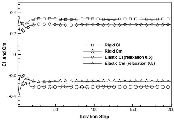
Fig. 5 History of  $C_l$  and  $C_m$  for different values of the relaxation parameter  $\alpha$ , Navier-Stokes computation
