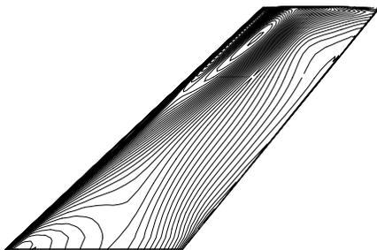
Fig. 10 Pressure contours on upper surface of rigid wing, Euler solution
