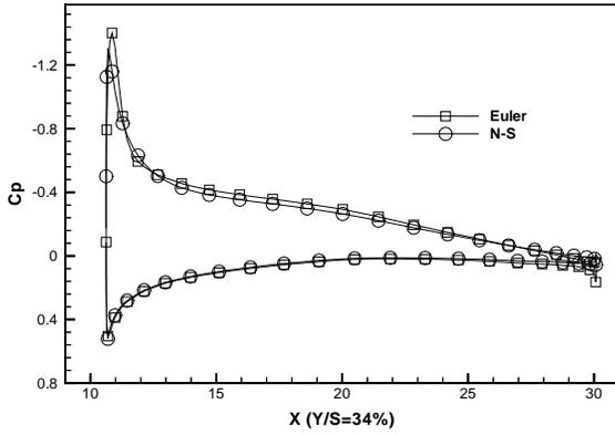
Fig. 8 Comparison of  $C_p$  distributions at 34% span by Euler and Navier-Stokes equations for the rigid wing
