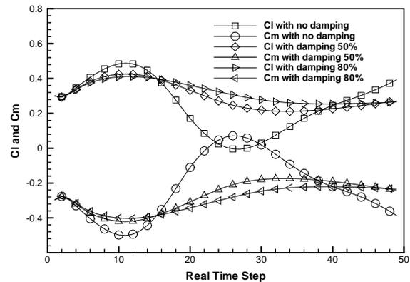
Fig. 3 History of  $C_l$  and  $C_m$  in time for different amounts of structural damping, Euler computation
