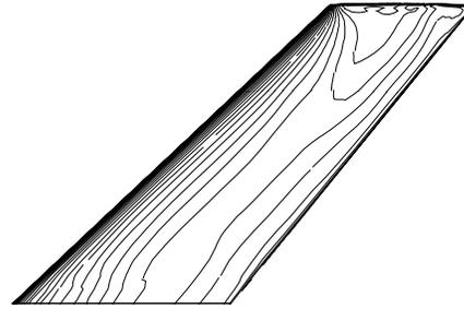
Fig. 17 Pressure contours on lower surface of elastic wing, Euler solution
