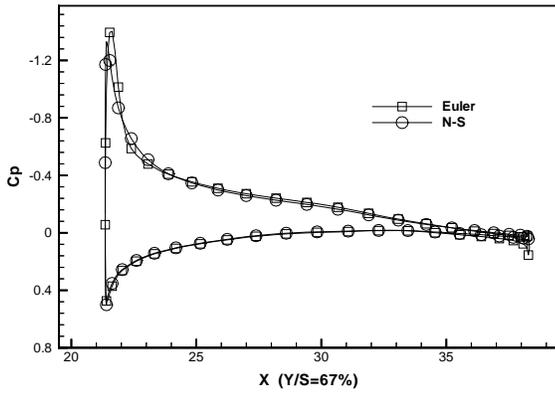
Fig. 15 Comparison of  $C_p$  distributions at 67% span by Euler and Navier-Stokes equations for the elastic wing
