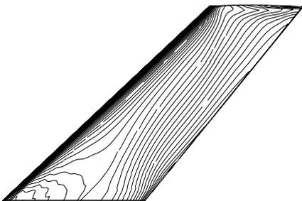
Fig. 16 Pressure contours on upper surface of elastic wing, Euler solution
