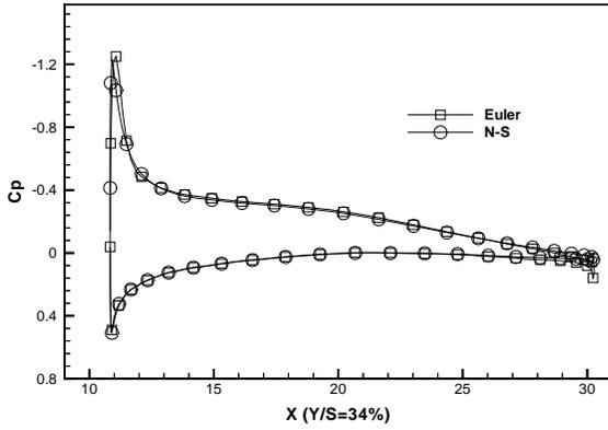
Fig. 14 Comparison of  $C_p$  distributions at 34% span by Euler and Navier-Stokes equations for the elastic wing
