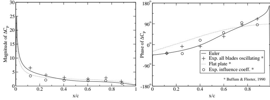
Figure 1. Unsteady pressure difference coefficient,  $IBPA = 0^\circ$ ,  $k = 0.223$
