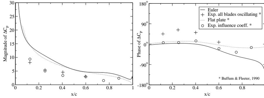
Figure 2. Unsteady pressure difference coefficient,  $IBPA = 90^\circ$ ,  $k = 0.223$
