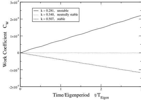
Figure 4. Total energy of the cascade over time at  $\mu = 450$
