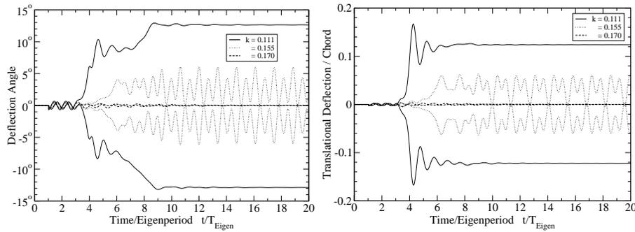
Figure 7. Bending + torsion: rotational and translational deflection over time
