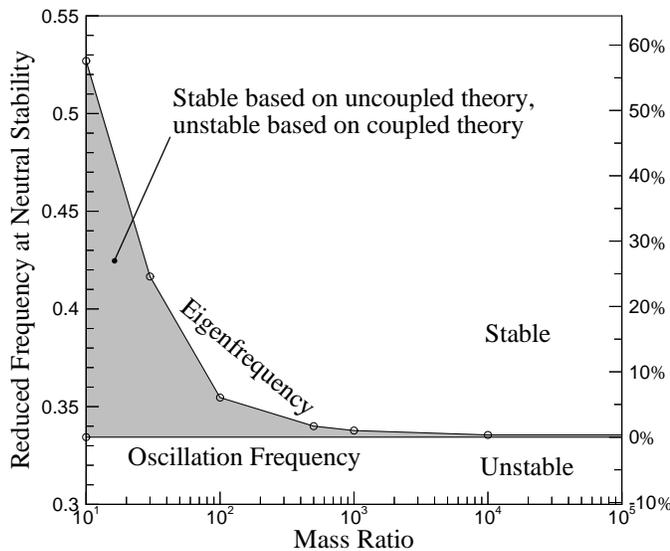
Figure 5. Frequency at neutral stability over mass ratio
