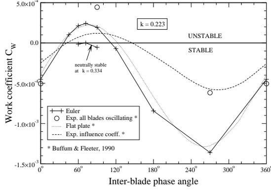
Figure 3. Work coefficient,  $k = 0.223$
