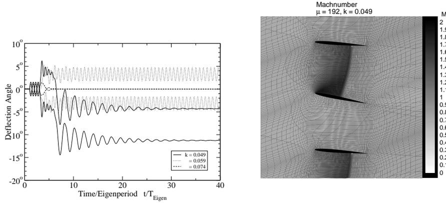
Figure 6. Pure torsion: rotational deflection over time, and Mach number distribution for  $k = 0.049$
