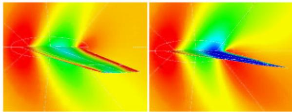
Pressure on The AGARD 1-Wing 445.6 (First Bending Mode and First Torsion Mode)
