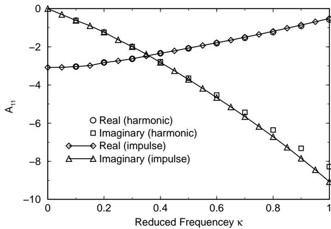
Figure 10: Comparison of generalized aerodynamic forces calculated by the harmonic and indicial methods  $Q_{11}$  for  $M_\infty = 0.901$
