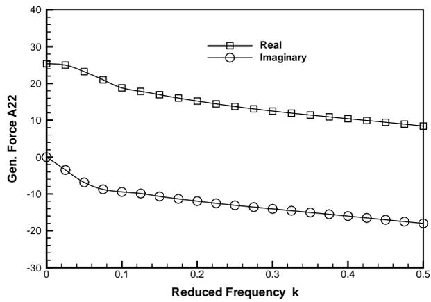
Figure 15: Generalized aerodynamic force  $Q_{22}$  for  $M_\infty = 0.960$
