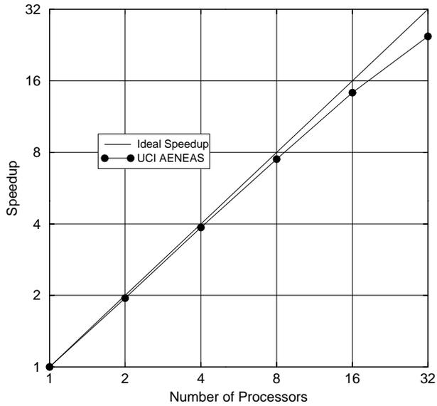
Figure 1: Parallel Speedup for the Parallel Unsteady NSAERO Code on a 32 node PC Cluster with 100Mb Switched Ethernet, 71001 grid points
