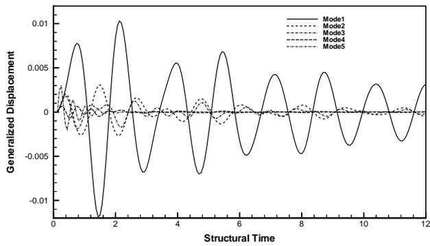
Figure 16: Time history of the generalized coordinates for the AGARD 445.6 wing for  $M_\infty = 1.141$  and  $V_f = 0.58$ .
