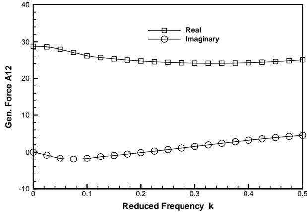
Figure 13: Generalized aerodynamic force  $Q_{12}$  for  $M_\infty = 0.960$
