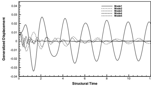
Figure 19: Time history of the generalized coordinates for the AGARD 445.6 wing for  $M_\infty = 1.072$  and  $V_f = 0.46$ .
