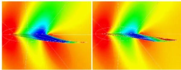
Pressure on The AGARD 1-Wing 445.6 (2nd Bending Mode and 2nd Torsion Mode)
