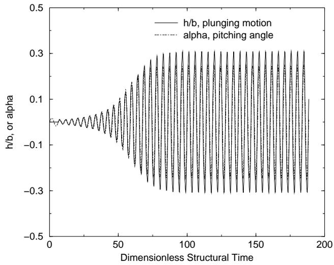
Figure 6: Time history of pitching and plunging motion for the Isogai wing model for  $M_\infty = 0.75$ , and  $V_f = 1.33$
