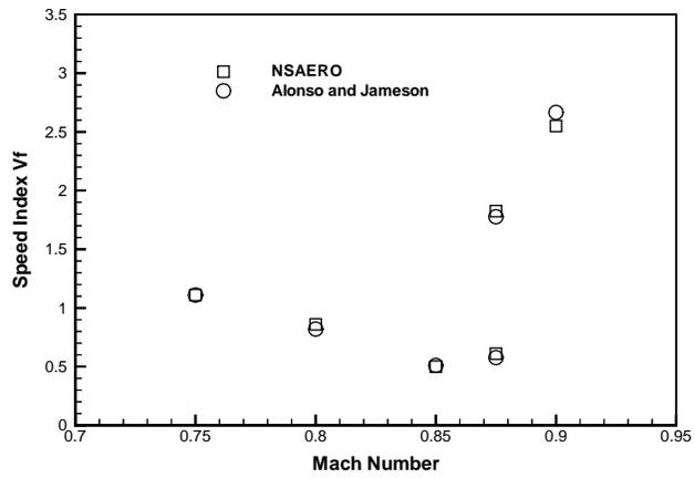
Figure 7: Flutter Boundary Predicted by NSAERO Compared to that by Alonso and Jameson[7]
