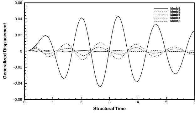
Figure 17: Time history of the generalized coordinates for the AGARD 445.6 wing for  $M_\infty = 1.141$  and  $V_f = 0.652$ .
