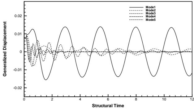
Figure 20: Time history of the generalized coordinates for the AGARD 445.6 wing for  $M_\infty = 0.901$  and  $V_f = 0.34$ .
