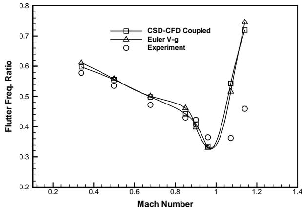
Figure 22: Flutter frequency for the AGARD 445.6 Wing.
