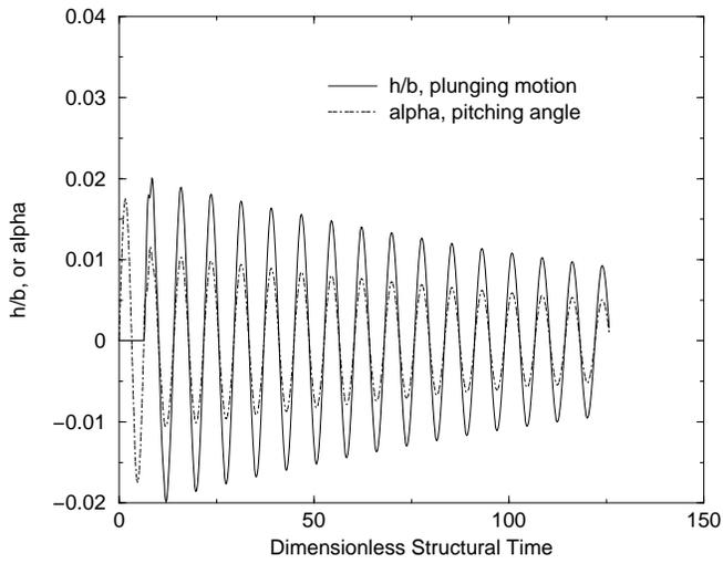
Figure 3: Time history of pitching and plunging motion for the Isogai wing model for  $M_\infty = 0.825$ , and  $V_f = 0.530$
