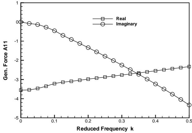
Figure 12: Generalized aerodynamic force  $Q_{11}$  for  $M_\infty = 0.960$
