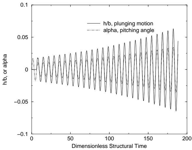
Figure 4: Time history of pitching and plunging motion for the Isogai wing model for  $M_\infty = 0.825$ , and  $V_f = 0.725$
