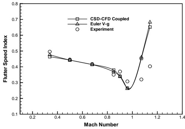
Figure 21: Flutter speed for the AGARD 445.6 Wing.
