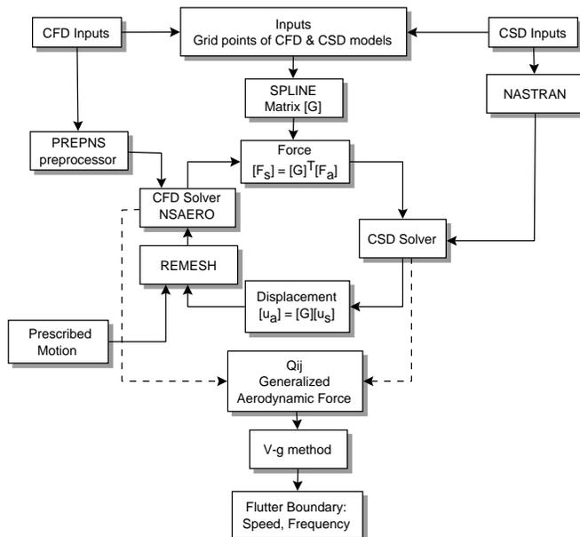
Figure 2: Integrated CFD-CSD Method for Flutter Calculations
