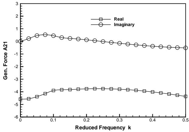
Figure 14: Generalized aerodynamic force  $Q_{21}$  for  $M_\infty = 0.960$
