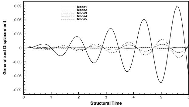
Figure 18: Time history of the generalized coordinates for the AGARD 445.6 wing for  $M_\infty = 1.141$  and  $V_f = 0.70$ .
