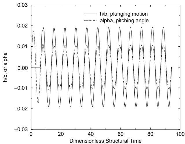
Figure 5: Time history of pitching and plunging motion for the Isogai wing model for  $M_\infty = 0.825$ , and  $V_f = 0.630$
