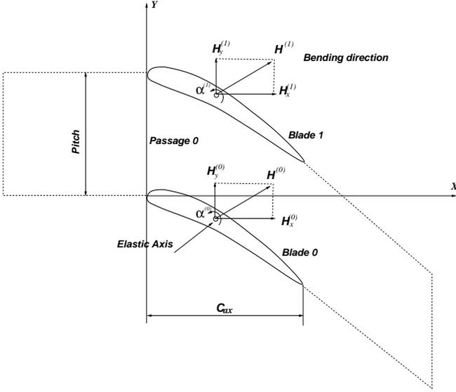
Figure 1: Blade geometry and motion definition
