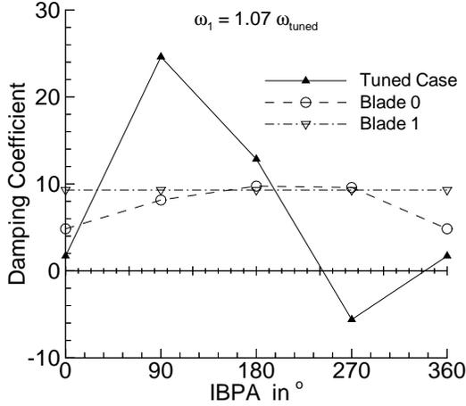
Figure 11: Damping coefficient vs. IBPA for blade 0 and 1. Blade 1 is mistuned in frequency by +7%.
