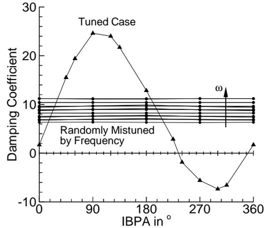
Figure 15: Damping coefficient for configuration shown in Figure 14.
