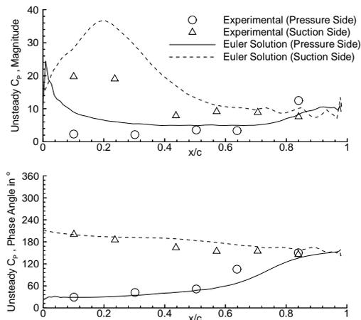
Figure 5: Amplitude and phase of the first harmonic unsteady pressure coefficient over the blade with  $IBPA = 180^\circ$
