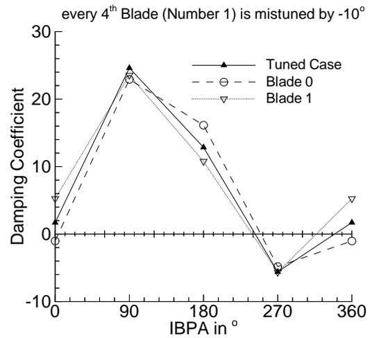
Figure 9: Damping coefficient vs. IBPA for blade 0 and 1. Blade 1 is mistuned in phase by  $-10^\circ$ .
