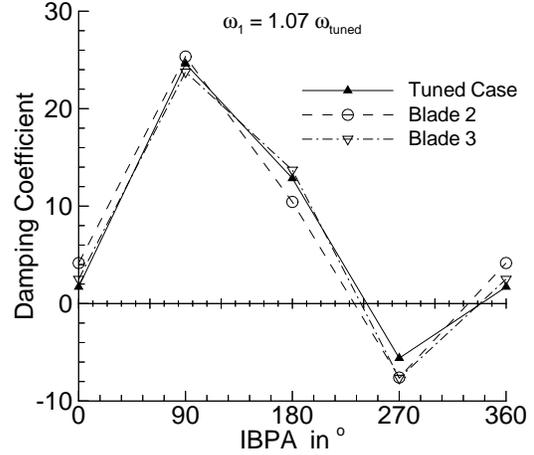
Figure 12: Damping coefficient vs. IBPA for blade 2 and 3. Blade 1 is mistuned in frequency by +7%.
