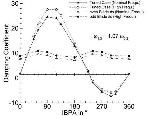
Figure 13: Damping coefficient vs. IBPA. Odd numbered blades are mistuned in frequency by +7%.
