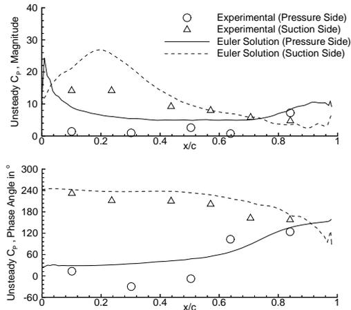
Figure 4: Amplitude and phase of the first harmonic unsteady pressure coefficient over the blade with  $IBPA = 90^\circ$
