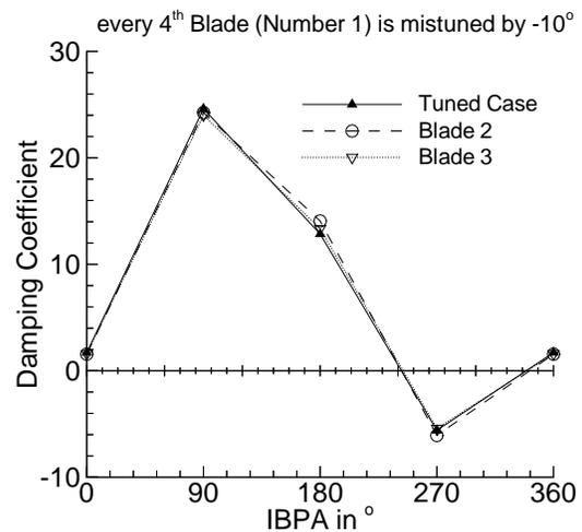
Figure 10: Damping coefficient vs. IBPA for blade 2 and 3. Blade 1 is mistuned in phase by  $-10^\circ$ .
