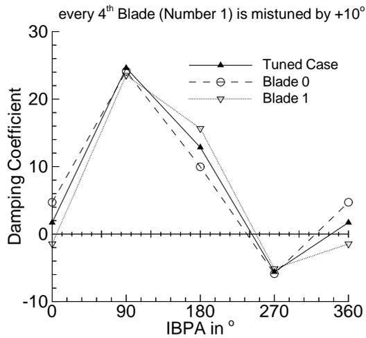
Figure 7: Damping coefficient vs. IBPA for blade 0 and 1. Blade 1 is mistuned in phase by  $+10^\circ$ .
