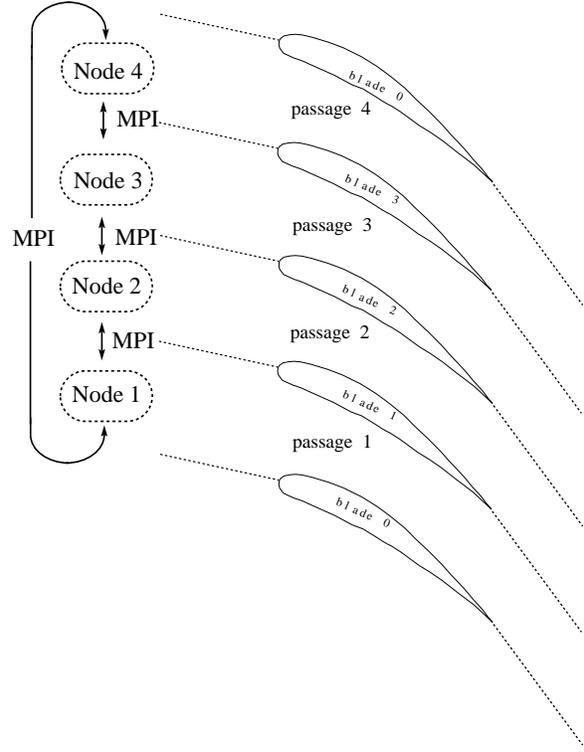
Figure 2: Multiple passage computation using MPI
