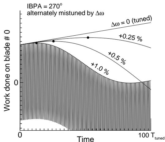
Figure 16: Work done on blade 0 vs. time, for various frequency differences.
