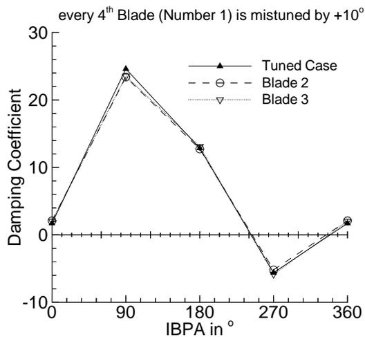
Figure 8: Damping coefficient vs. IBPA for blade 2 and 3. Blade 1 is mistuned in phase by  $+10^\circ$ .
